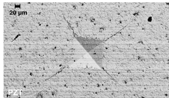
Fig. 2. Vickers indentation to measure fracture toughness.
